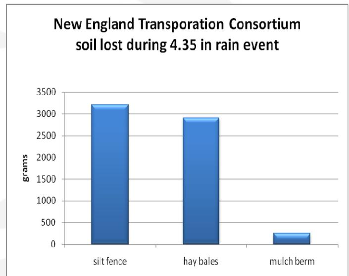
Figure 1. Sediment removal comparison (Source: Dumars et al, 2000)
